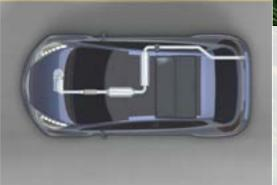
key enabler to Plug-in Hybrid Electric Vehicles (PHEV) architectures that need to regain underbody space to allow large battery packs.
