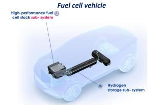
These two key elements are **hydrogen storage systems**, which the Group develops on its own, and **fuel cell stacks** produced by Symbio, the joint venture created with Michelin.
