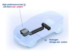
These two key elements are **hydrogen storage systems**, which the Group develops on its own, and **fuel cell stacks** produced by Symbio, the joint venture created with Michelin.
